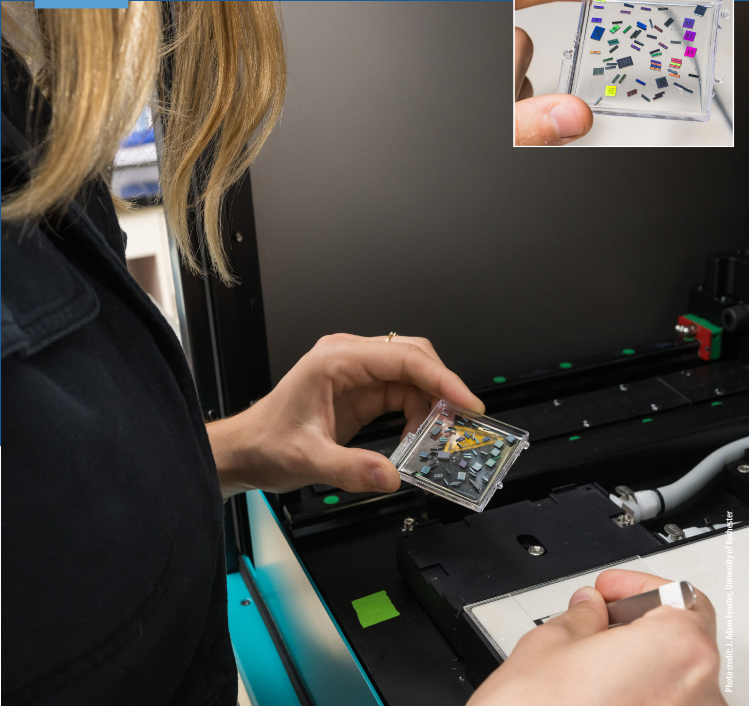
Biomedical engineering PhD student Katie Daniel loads photonic sensor chips into a printer to be functionalized with capture molecules in the lab of Professor Benjamin Miller.
