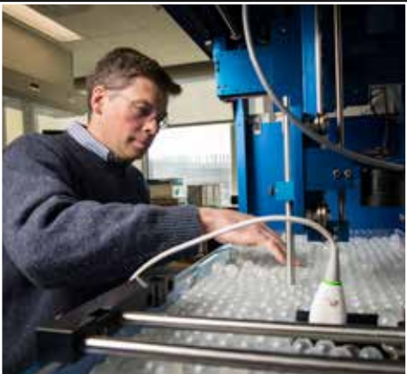
Stephen McAleavey, the chair of the biomedical engineering department and an associate professor of biomedical engineering and of electrical and computer engineering at the University of Rochester, is photographed in his lab with a tank used to measure the acoustic field of an ultrasound transducer, allowing for degassed and deionized water. Plastic balls (viewed from below in the large photo) prevent oxygenation of the water.
